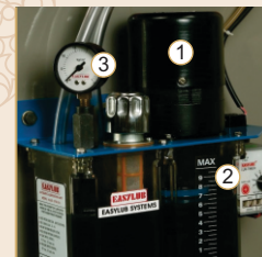
1 Motorized Auto Lubrication System 2 Electronic Timer 3 Oil Pressure Gauge
